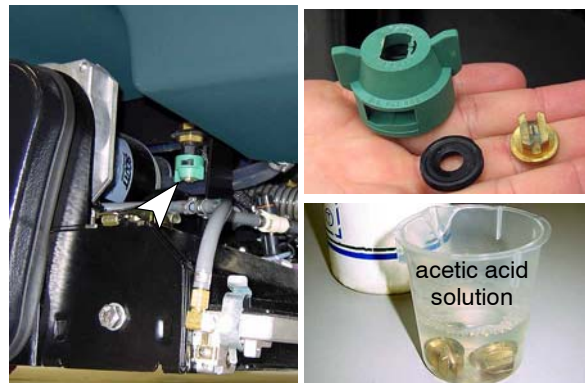
ReadySpace Spray Nozzle GREEN CAP / TIP #11002 p/n 575283000
